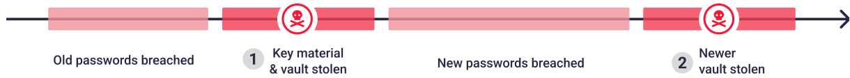
Figure 20: Without Post-Compromise Security new passwords generated after a device compromise are breached again when a newer vault is stolen.
