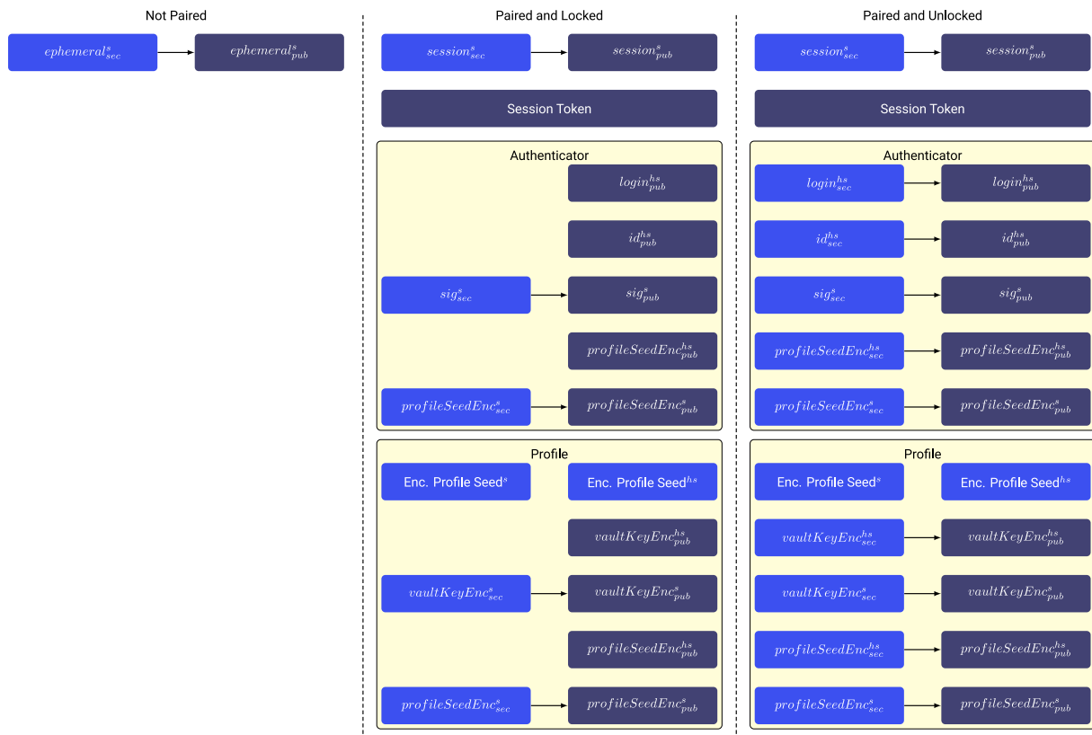
Figure 28: Different states of a client device and which keys are available to it.
